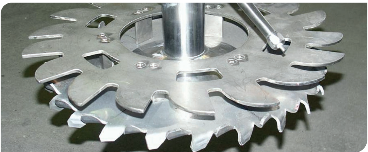
High performance dispersion via single shaft high speed dispenser and large double sucking disc Picture by WILHELM NIEMANN GmbH & Co., www.niemann.de
