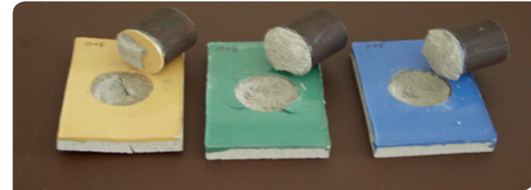
Picture 1: Adhesion on concrete surfaces
